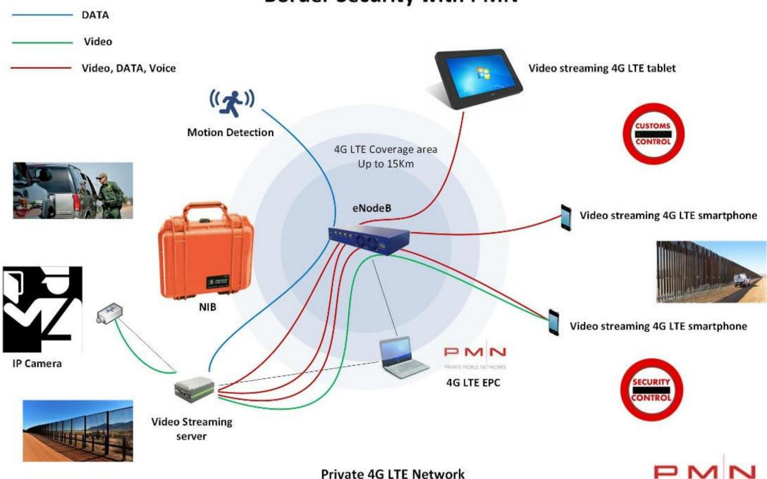
Network In a Box (NIB) (2G GSM, 3G UMTS, 4G LTE)
