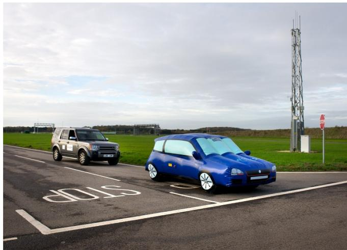
*Simulated rear end collision using dummy vehicle to test eCall operation*
