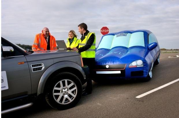
***Engineers interrogate the eCall system to confirm that the emergency call has been successfully routed to an external Public Service Access Point (PSAP) from innovITS ADVANCE***
